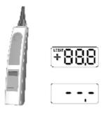
A short sound signifies the measuring cycle (approximately four seconds) is finished. At least 4 of 10 impulses must be accepted in order to get a valid reading. A valid reading is shown on the display. If less than 4 impulses were valid, no reading will be indicated on the display. The display will show - - . - .
